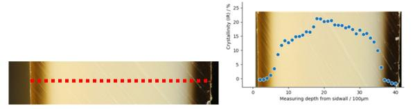
Step 5. Spectral analysis of the IR line scans was conducted to derive crystallinity profile. Spatiallyresolved quantification of crystallinity via IR band evaluation
