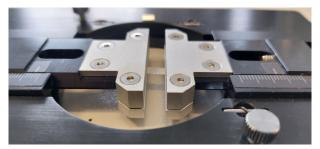
Step 3. Setting the MicroVice Holder with the mounted sample onto the stage of the IR microscope
