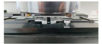
Step 4. IR line scans were performed along the cross-section of the microtome cuts
